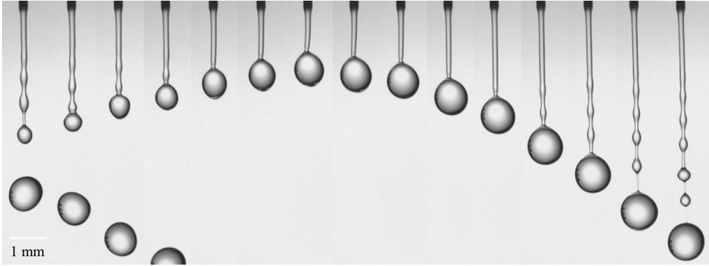
FIGURE 1. The ‘gobbling’ phenomenon: a large terminal drop periodically develops at the end of a thin jet of a viscoelastic fluid (100 ppm PAA solution, Q = 39.7 \text{ mm}^3 \text{ s}^{-1} , R_i = 0.125 \text{ mm} ). A sequence of video images is shown; the time interval between consecutive images is 6 ms.
